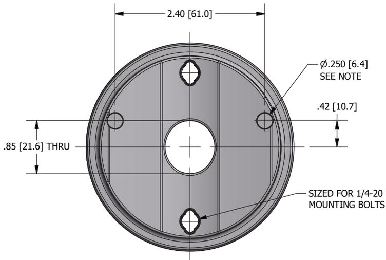
This cast aluminum Universal Bulldog Pole Mount is uniquely designed to provide either: a very strong and low profile mounting option for Polara's Bulldog Push Button, or as an adapter to a variety of existing mountings. With Polara's Bulldog Button attached to this mount (and directly to the pole), the main body of the button extends only 1.5" from the pole.
