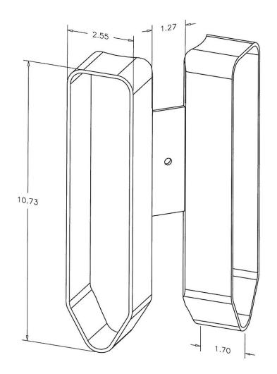
This spacer is designed to offset two Push Button Frames on a 4.5" diameter pole so that two 9" x 12" signs can be mounted without conflict. One spacer is used to mount two Push Button Frames. The spacer is held to the pole by a bolt in the center and the frames mount to the pole with 3" long bolts through the spacer.
