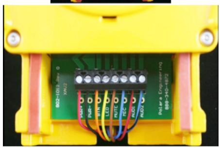
Press any excess wire into the cavity above terminal block or route the excess wire back into the pole. Make sure the wires are within the guide channel of the PBS (not pinched between pole and PBS), then tighten the two bolts until the PBS is secure on the pole. Install the bottom cover by securing the two screws on the bottom of the unit. Reinstall the sign making sure hand symbol points in same direction as arrow on button.
