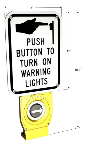
The XAV2E-LED push button station is designed for use at a pedestrian crosswalk with in-pavement or overhead flashing yellow lights. It works in conjunction with the XAVCU2 control unit. Within this system, the XAV2E-LED provides a 9X12 instructional sign, a push button with directional arrow for activating the flashing lights, a voice message, and a group of three yellow LEDs above the push button which flash in sync with the street lighting.
