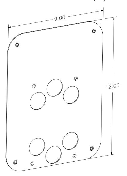
Polara Engineering's 9" x 12" Push Button Frame Adapter is designed to be attached to Polara's PBF5X7-X Push Button Frame, for mounting 9" x 12" crosswalk signs. These adapters can also be used on 2 wire and 4 wire Navigators. Their aluminum structure and powder coat finish provides a very strong and attractive mount for crosswalk signs.
