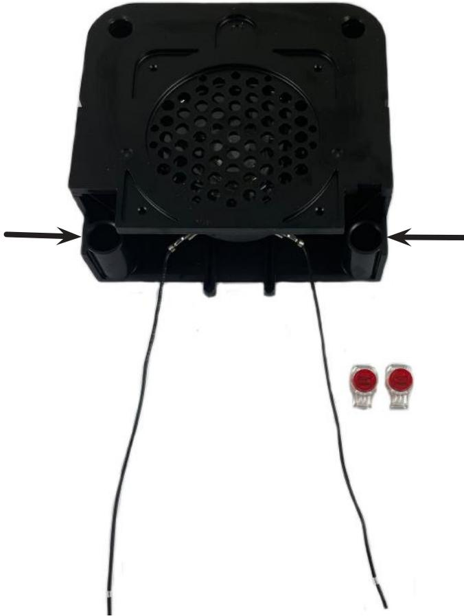
The iNS-SPKR is a field replacement speaker module for an iNS (iNavigator S) Push Button Station (PBS).
